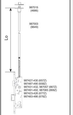
Bolt length measured without sliding stopper and without connector thread.
